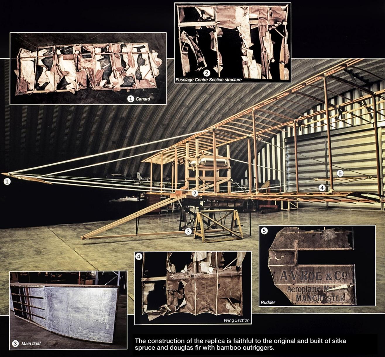
The original had a take-off run of 75 yards, lift-off at 32 miles per hour, and flying speed between 45 and 50 miles per hour.
